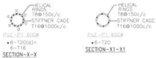
TYP SECTIONAL ELEVATION OF PILE-P1
